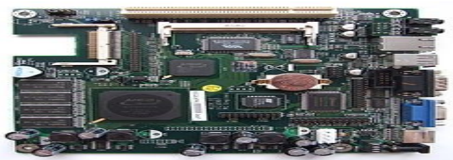
Fig3: PC Engines' ALIX.1C Mini-ITX embedded board with an x86 AMD Geode LX 800 together with Compact Flash, miniPCI and PCI slots, 44-pin IDE interface, audio, USB and 256MB RAM
